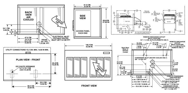
INSTALLATION NOTE: Allow 6" minimum space at back for ventilation and utility connections.
